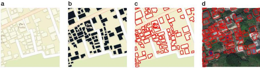
**Figure 4.2.** Process of extracting buildings from an ESRI WMS image.
