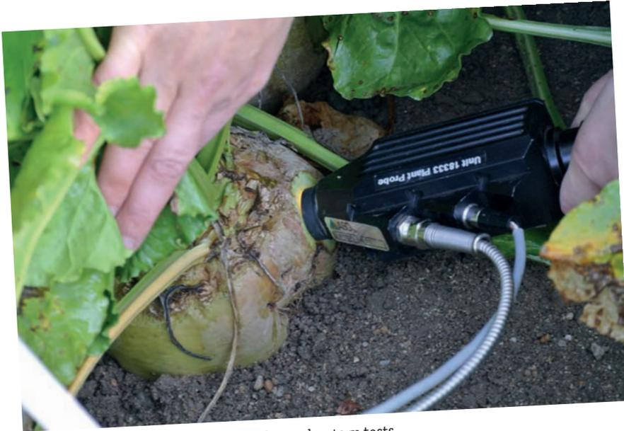
Plant probe (ASD) used for the exploratory tests of the sugar content measurement.
