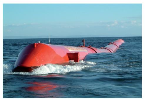
■ Photo 32 : Pelamis system to recover wave energy being tested under smooth conditions at the European Marine Energy Centre in Scotland (© Pelamis Wave Power Ltd, UK).
