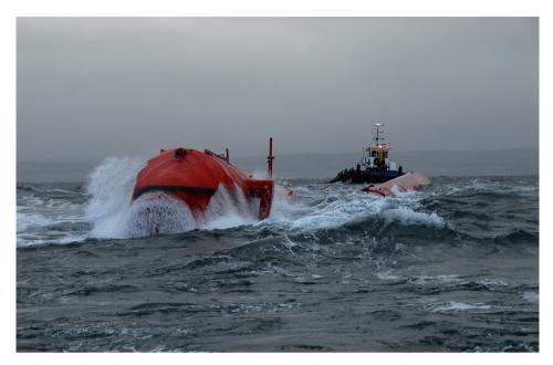
■ Photo 1 : the Pelamis system to recover wave energy being tested under rough conditions at the European Marine Energy Centre in Scotland (© Pelamis Wave Power Ltd, UK).
