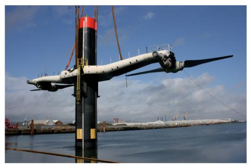
■ Photo 30 : Seagen stream turbine installed at Strangford Narrows in Northern Ireland (© Marine Current Turbines Ltd, UK).
