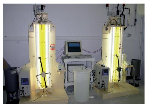
■ Photo 34 : photobioreactors holding 17 litres used to feed the bivalve mollusc larvae and juveniles (© Ifremer, J.P. Cadoret).
