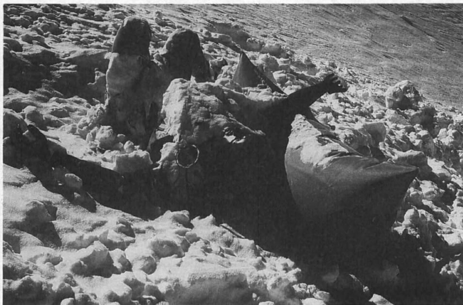
Fig. 2: Test dummy with ABS balloon on the avalanche deposit
